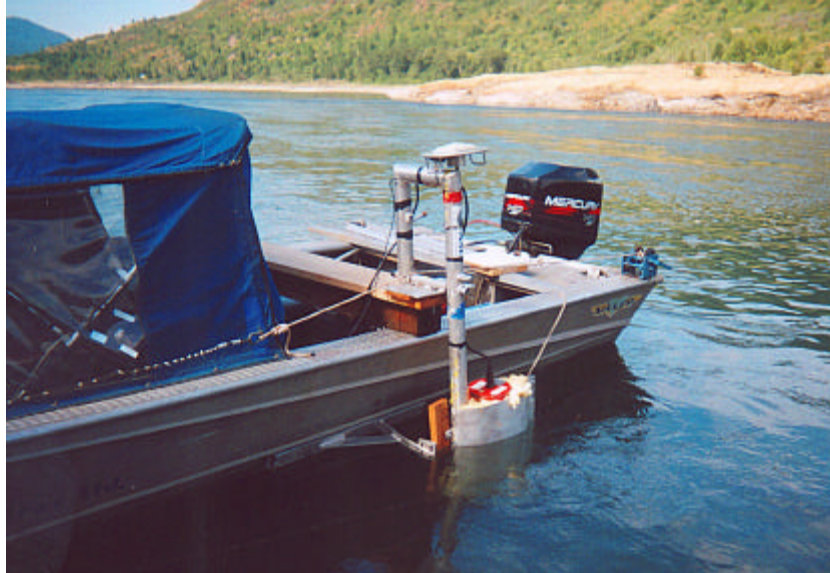
Figure 3: The acoustic doppler current profiler flow meter attached to an aluminium work boat used for flow surveys.
