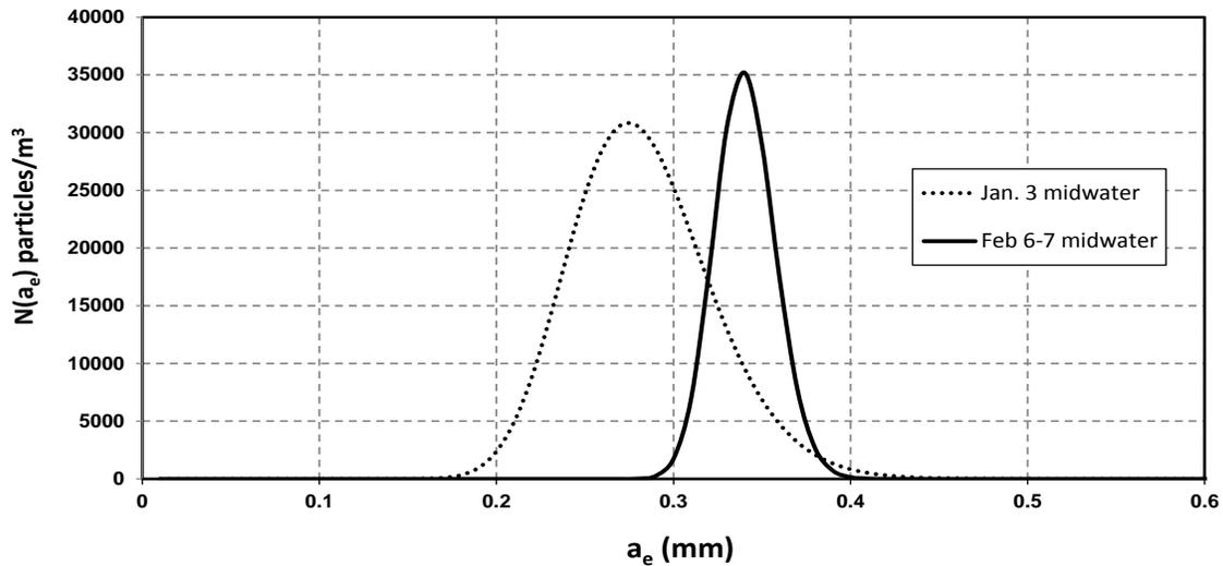
**Fig. 6.** Numbers of particles per  $m^3$  as at midwater (2.3 m) ranges for the Jan. 2-3 and Feb. 6-7 frazil study intervals.
