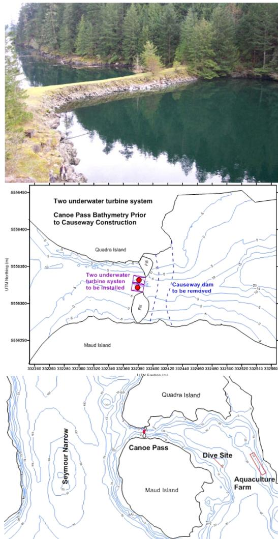
**Figure 6: The existing Canoe Pass causeway (upper); the locations of the two underwater turbines in place of the causeway (middle) and the locations of the Dive site, Aquaculture farm and the Seymour Narrows navigation channel**
