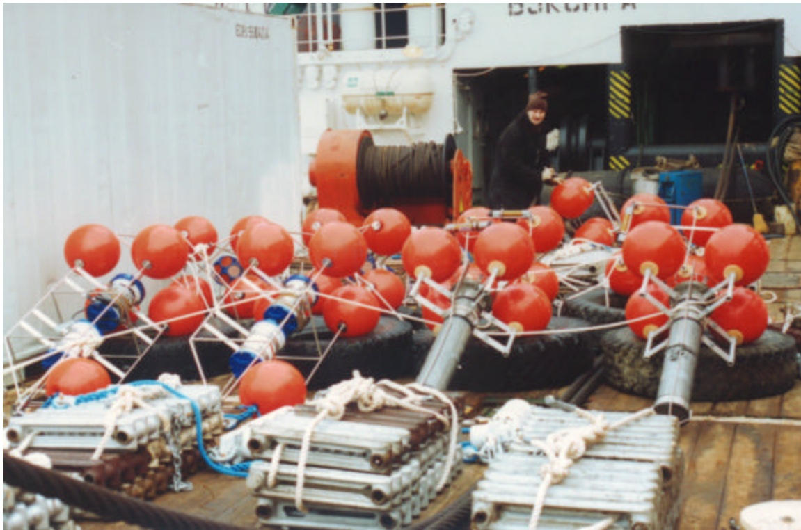
Figure 1. IPS4 and ADCP moorings laid out on the stern of the vessel “Neftegaz ‘70” in preparation for deployment.
