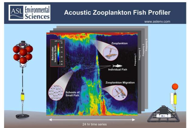
Acoustic Zooplankton Fish Profiler (AZFP) data time series and example mooring configurations.
