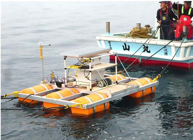
Test mooring of raft-mounted AZFP equipped with cellular modem used to study zooplankton in the water column, Yamada Bay, Japan, June 2016. Note that, in subsequent tests, the solar panel array was modified and expanded.
