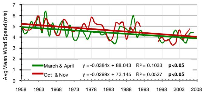
Figure 4. Wind speed (m/s) trends at Tuktoyaktuk NWT calculated as the average of the mean wind speed for March-April, and October-November.
