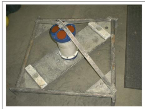
**Golder Associates** of Edmonton, Alberta leased a 300kHz RDI ADCP for measurements related to a mine and jetty development in Nunavut. ASL also provided a bottom frame that could be deployed from their small boat.
