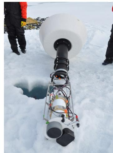
AZFP zooplankton sensor in its frame, attached to the buoy hull before deployment next to the prepared deployment hole in the sea ice. Photo by Dr. Lovro Valcic.
