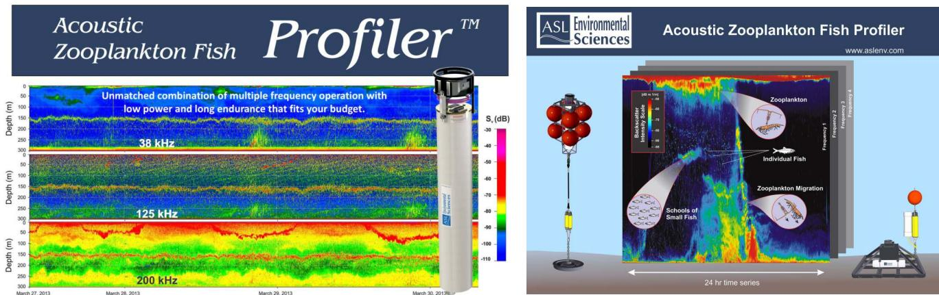
Acoustic Zooplankton Fish Profiler (AZFP) data time series and example mooring configurations.
