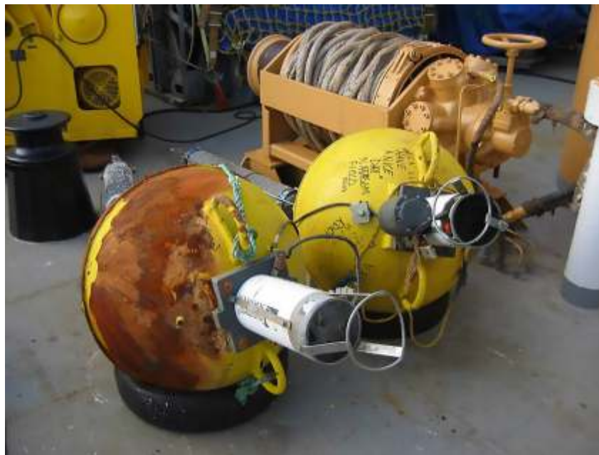
The two IPS4 units which were struck by the ice island on September 22, 2010 as seen following recovery in 2012. Besides the bent transducer guards, no significant damage was sustained.
