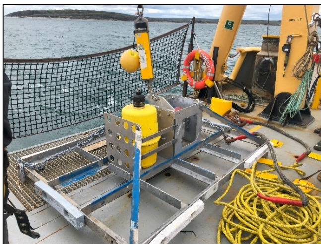
ADCP mooring prepped for deployment (top). Mooring recovery off the aft of the RV Coriolis (bottom).
