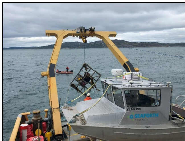
ADCP mooring prepped for deployment (top). Mooring recovery off the aft of the RV Coriolis (bottom).
