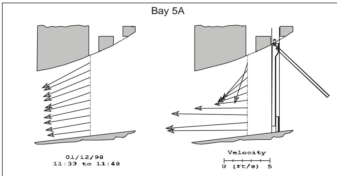
**Figure 3: Flow vectors measured in the intake, without ESBS screens (left) and with screens (right).**
