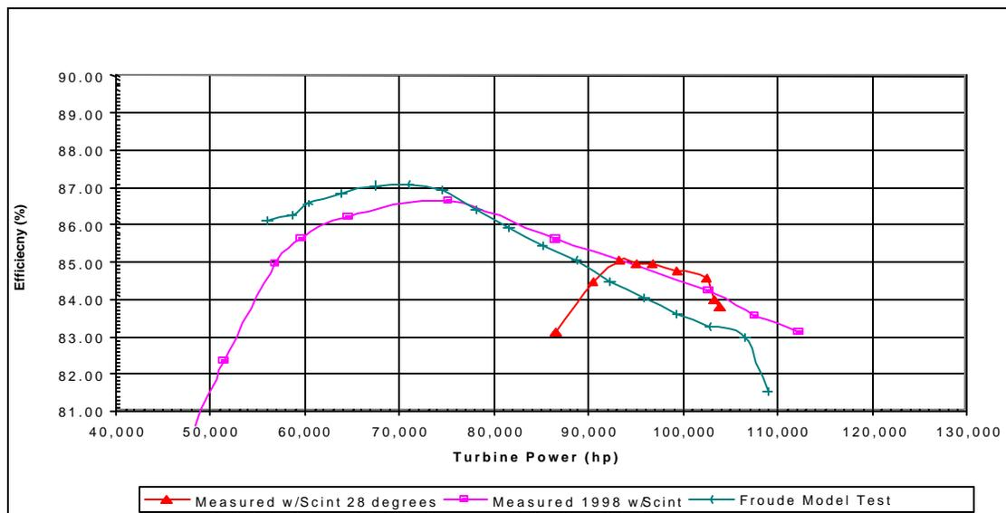
**Figure 7: Froude Model Predicted Prototype Performance With ESBS Screens Compared to Field Measured Performance Using Scintillation Flow Measurements.**
