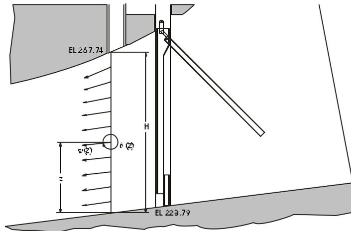
**Figure 2: Location of the measurement plane in the intake, and definition of associated parameters.**
