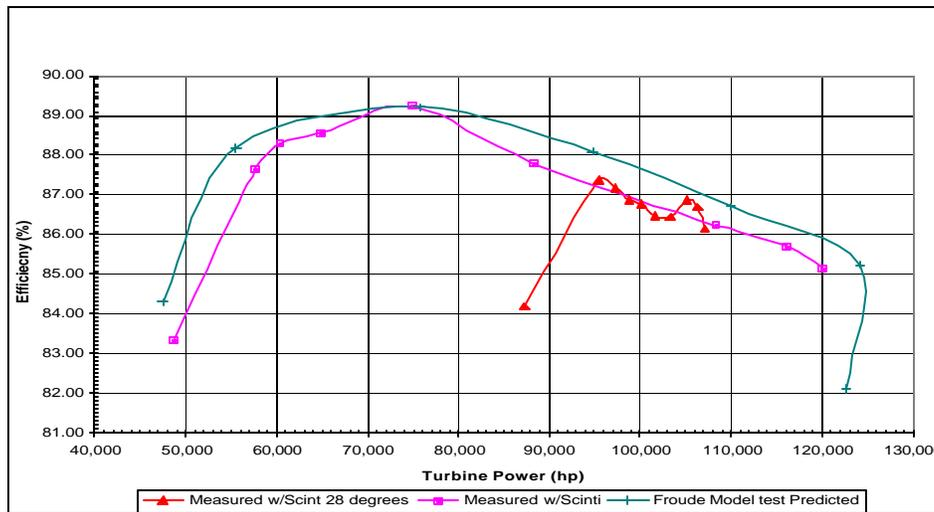
**Figure 6: Froude Model Predicted Prototype Performance With No Screens Installed Compared to Field Measured Performance Using Scintillation Flow Measurements.**
