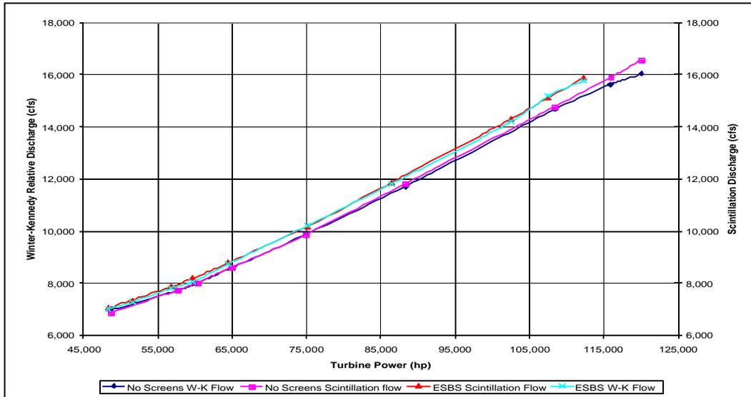
**Figure 5: Comparison of ASFM flow measurements to Winter-Kennedy Differential Pressure Relative Flow Measurements Without Fish Screens and with ESBS Screens Installed.**
