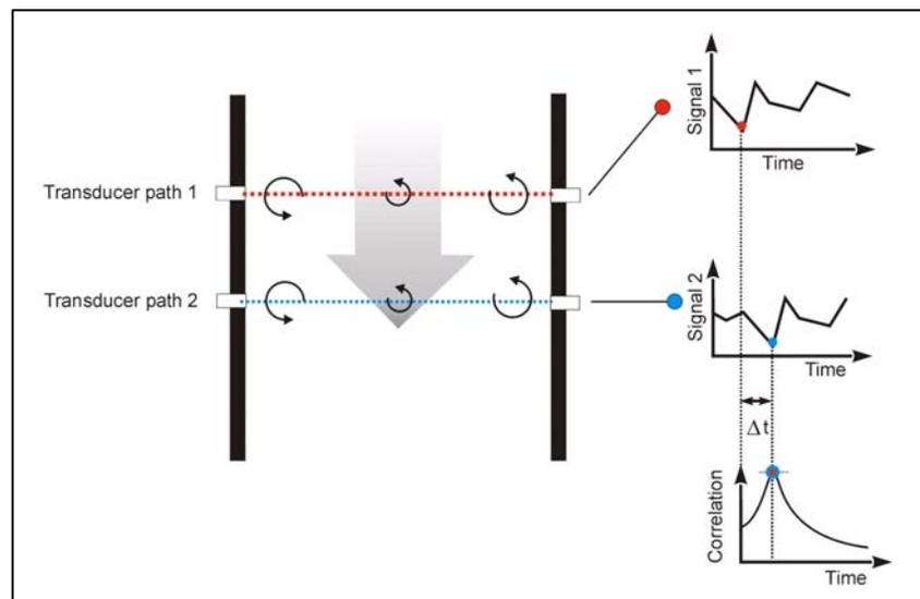
**Figure 1 - Illustration of acoustic scintillation drift principle**
