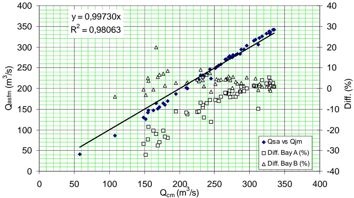
**Figure 4- Comparison of discharge measurement by CM and ASFM at Rocher-de-Grand-Mère, original data**
