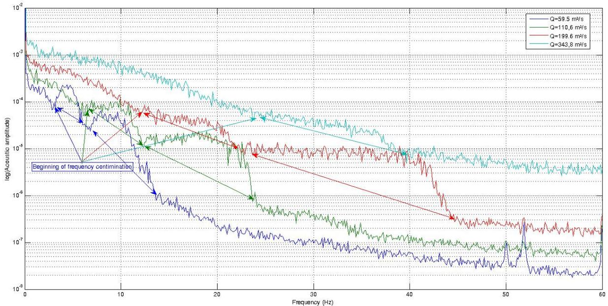
**Figure 6- Spectral analysis of the acoustic amplitude**
