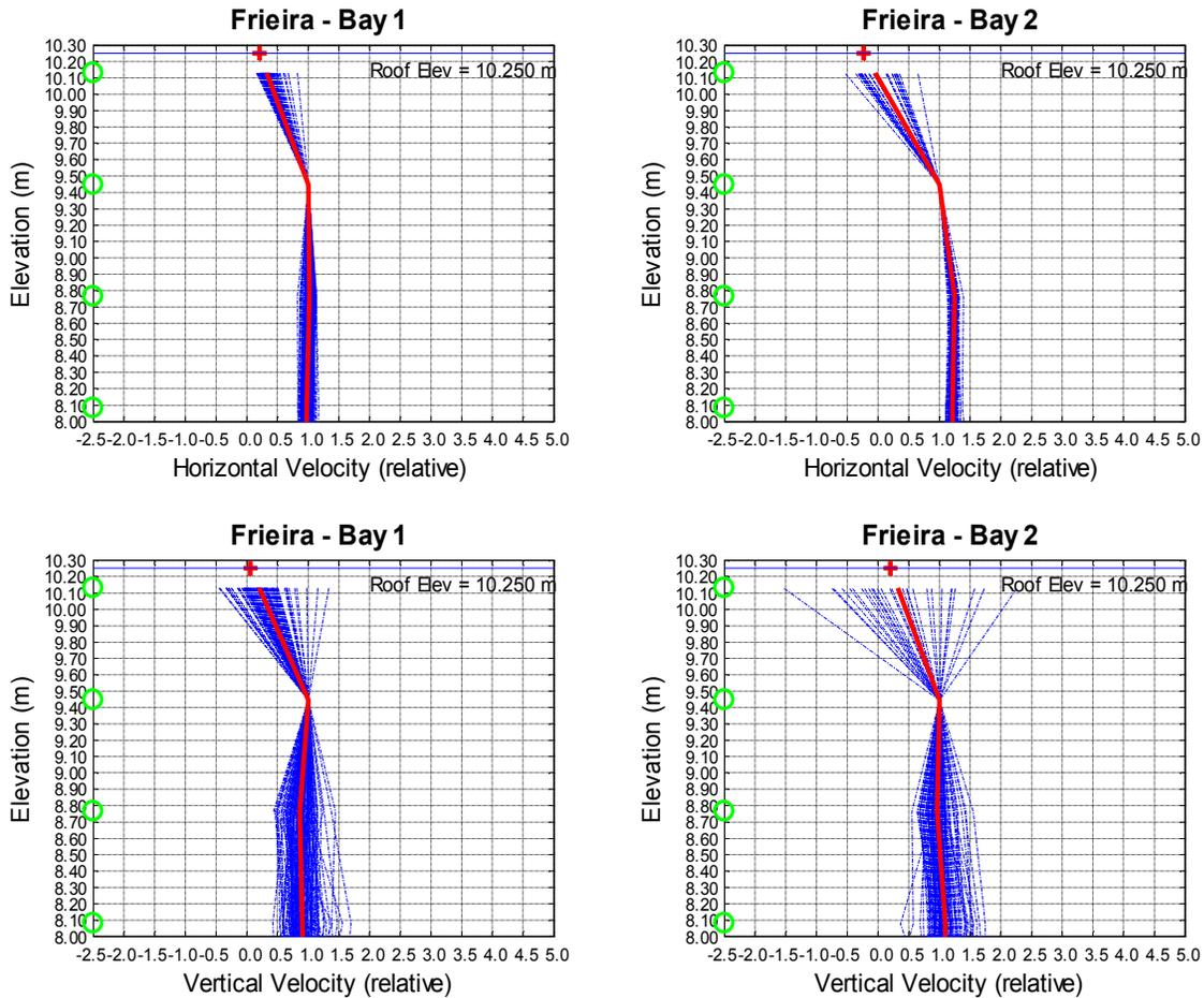
**Figure 9: Measured relative horizontal velocity (top) and vertical velocity (bottom) at Frieira**
