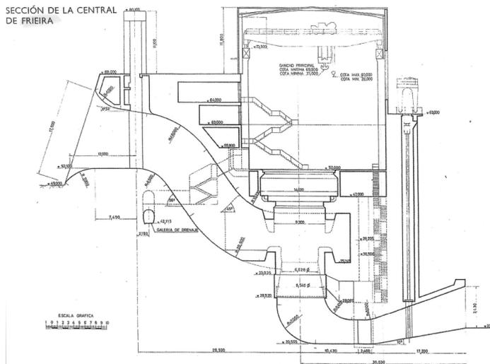
Figure 2: Schematic of the intake bays at the Frieira plant
