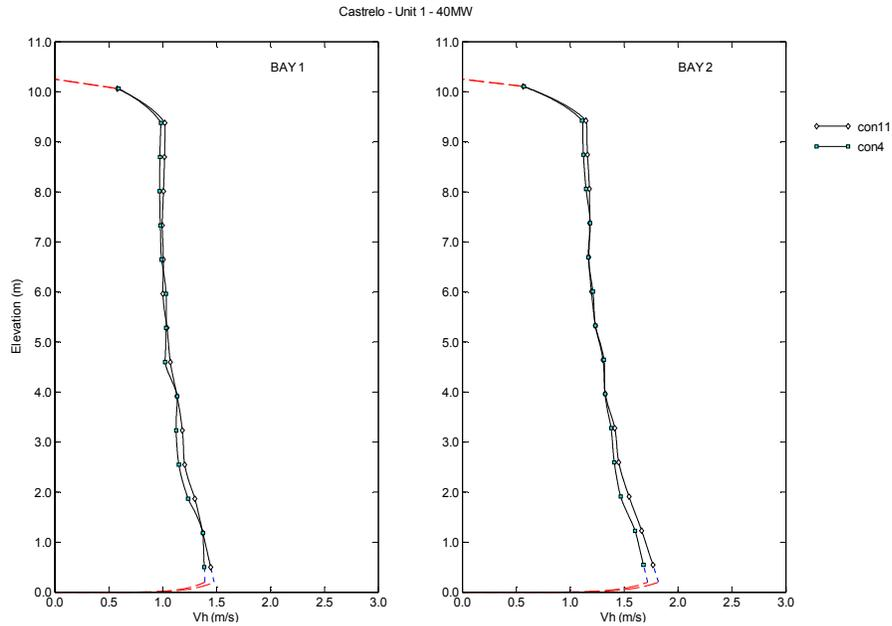
**Figure 10: Plots of the horizontal component of velocity at Castelo (40 MW).**
