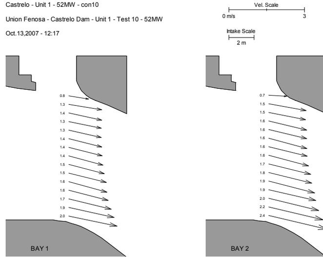
**Figure 8: Sample velocity vector plot from Unit 1 at Castrelo**
