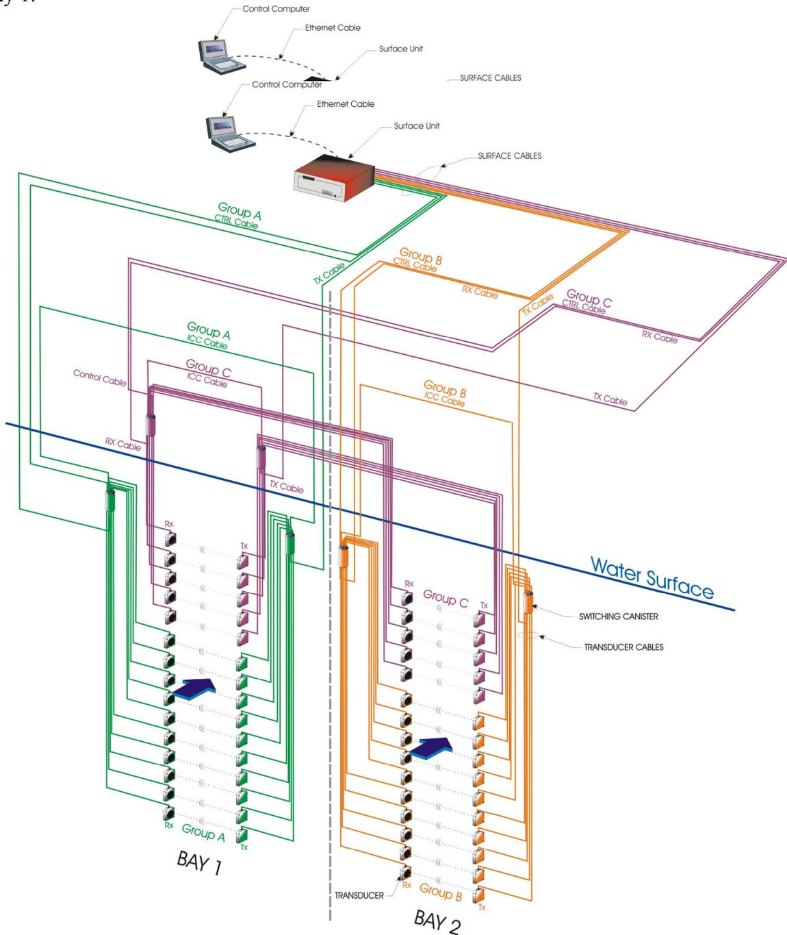
Figure 7: Components of the 2-bay, 15-path ASFM system. The arrows indicate the flow direction
