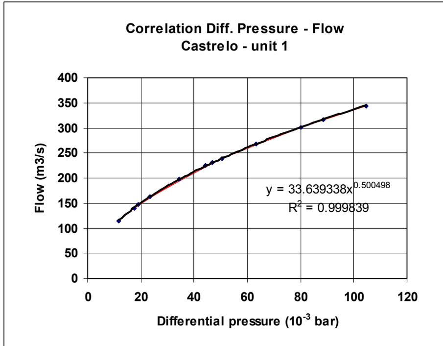
Figure 13: Flow comparison for Unit 1 at the Castrelo plant
