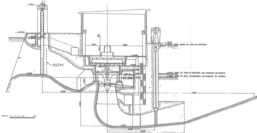
Figure 1: Schematic of the intake bays at the Velle plant
