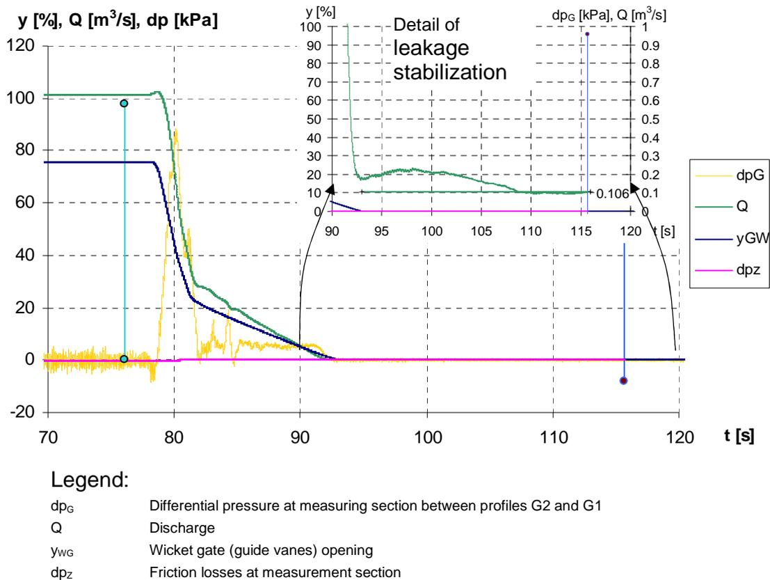
Fig. 3 – Example of pressure-time diagram
