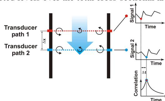
*Fig. 4- Representation of the acoustic scintillation principle*
