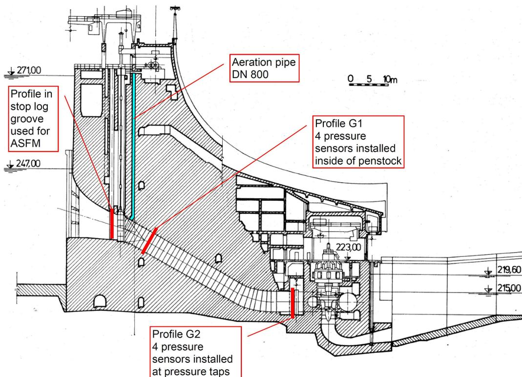
*Fig. 1 – Longitudinal section of HPP Slapy*
