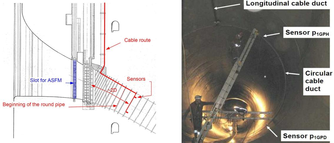
*Fig. 2 - Upper part of the penstock with pressure sensors in upstream profile*
