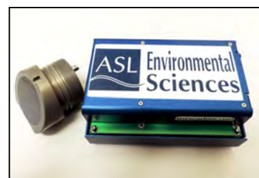
Figure 2: Angled 200kHz transducer for ECOPuck glider hull and AZFP electronics
