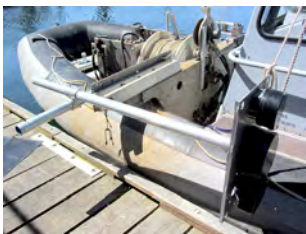
Figure 2: The transducer mount swivels to allow the transducers to be lifted out of the water
