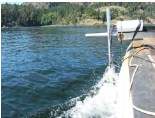
Figure 3: Collecting data at 4 knots (7.5 km/hr) without interference from bubbles
