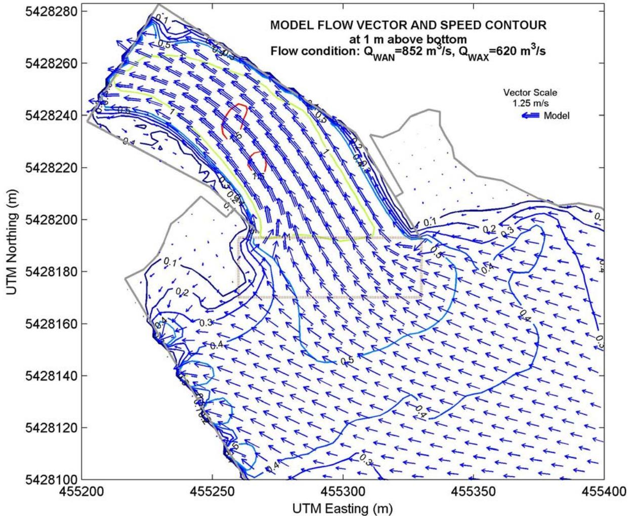
Figure 10: Model results of the headpond velocities at 1 m above bottom for a case with an existing Waneta turbine discharge of 852 m<sup>3</sup>/s and a WEP turbine discharge of 620 m<sup>3</sup>/s.
