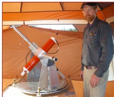
ASL compass calibration of a DVS 750 in the arctic during summer 2009.
