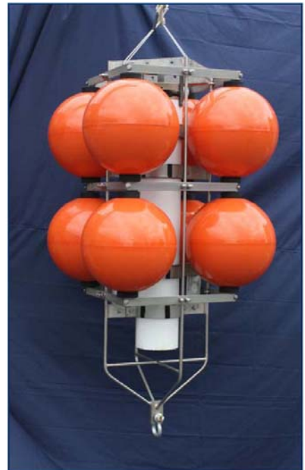
The dual cage with the ASL Ice Profiler or Acoustic Zooplankton Fish Profiler
