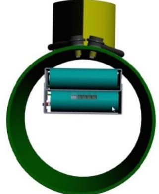
Rear view of the electronics package and transducer fairing mounted on a glider body (shown with optional internal Lithium battery pack).
