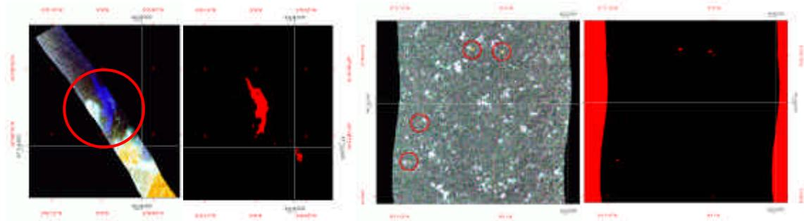
**Figure 7.** Mapping results: original images and detection maps. (Left) Large oil slicks; (Right) Scattered small oil slicks.
