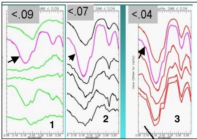
Figure 1 – Spectra extracted from Low Altitude AVIRIS alunite image over the Dragon Mine, UT. The best matches to the reference spectrum (marked with an arrow) are seen in [3], with
