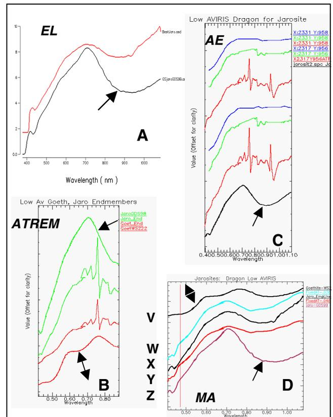
Figure 2– Spectra extracted from the Low Altitude AVIRIS iron mineral image over the Dragon Mine, UT. Reference spectra are flagged with an arrow for jarosite and double arrow for goethite. [A] Empirical Line spectra for jarosite, [B] standard ATREM corrected spectra for jarosite and goethite, [C] ATREM/EFFORT corrected spectra for jarosite, and [D] Modified ATREM corrected spectra for goethite and jarosite.
