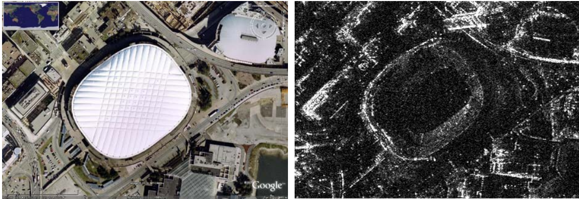
Figure 8: BC Place, Vancouver, Canada. GoogleEarth image of BC Place dome (left) and see-through capability of high resolution SAR image, TerraSAR-X (right).
