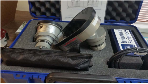
Figure 2 38 kHz transducer and 125/200 kHz transducer
