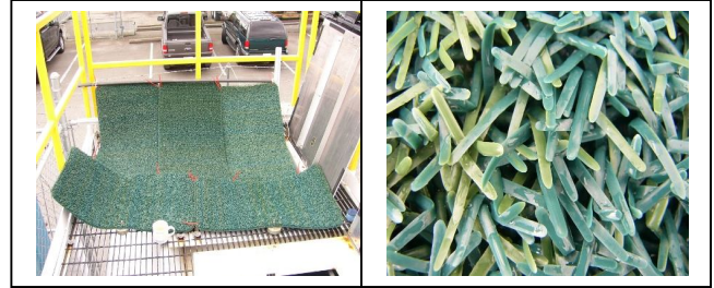
Figure 4. (a) Artificial turf used for sound absorption. (b) Diagram at the right shows a close up of the turf "shag"
