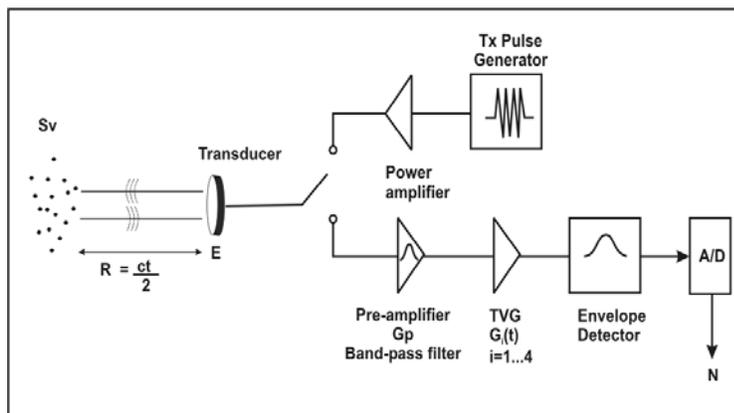
**Figure 1.** The generalized signal path for an Acoustic Water Column Profiler.
