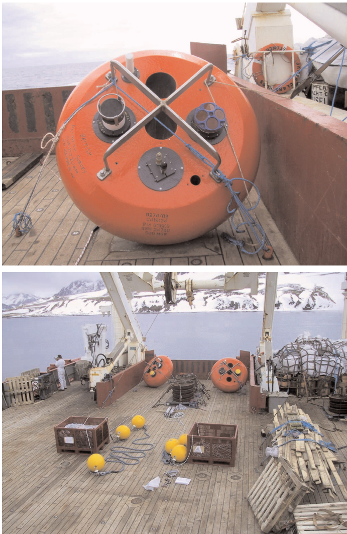
Fig. 2. Photographs showing (a, upper panel) the mooring buoyancy float and instruments (ADCP right, WCP left, Argos beacon top, radio and light beacons bottom; the CTD is beneath the float and hence not visible) and (b, lower panel) both moorings on the afterdeck of RRS James Clark Ross (the off-shelf mooring is on the lefthand side, and has substantially more tether in the square basket than does the on-shelf mooring). The instrument floats, railway-wheel ballast, and acoustic releases are lying beneath the A-frame.
