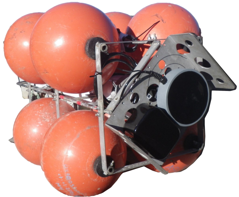
AZFP-ice deployment configuration. The black circular transducer is for the ice profiler and the black square transducer is for the multi-frequency calibrated echosounder.
