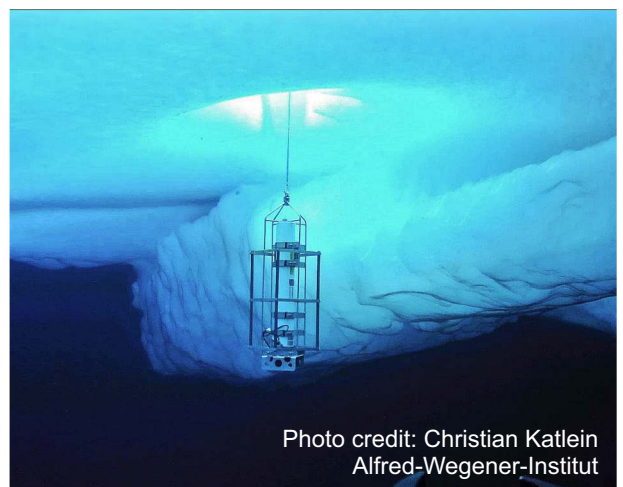
Ice-tethered AZFP deployment under multi-year sea ice in the Canadian high Arctic.
