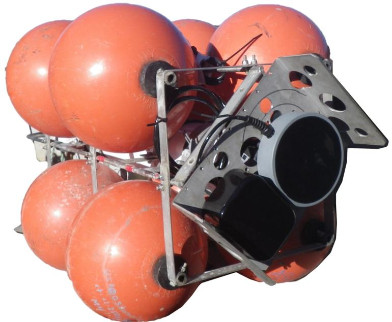
AZFP6-ice deployment configuration. The black circular transducer is for the ice profiler and the black square transducer is for the multi-frequency calibrated echosounder.
