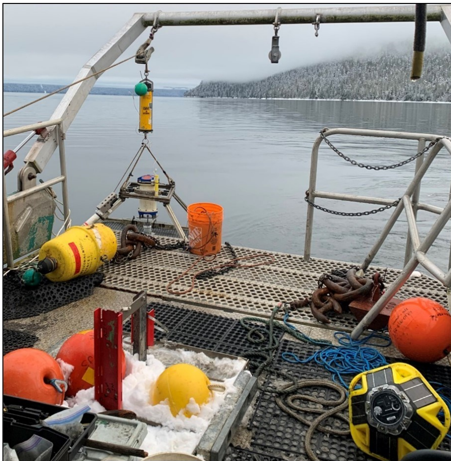
ADCP in bottom frame ready for deployment. A Spotter wave buoy (lower right) was also used for part of the study.
