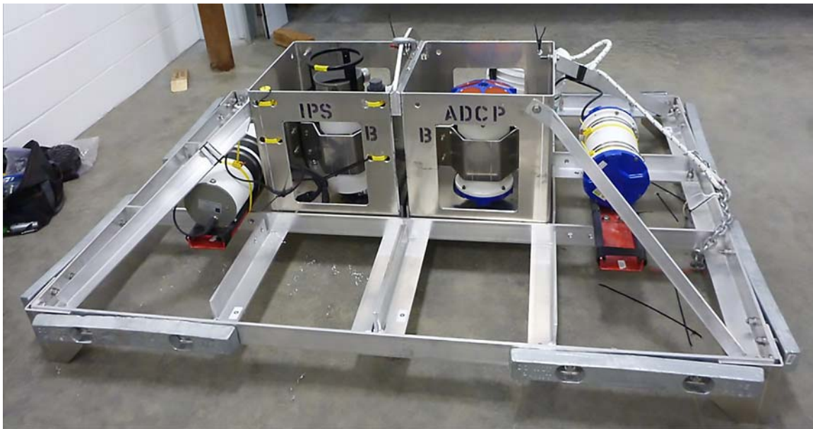
Figure 1: ASL trawl resistant LowPro5x7™ IceProfiler™/ADCP mooring
