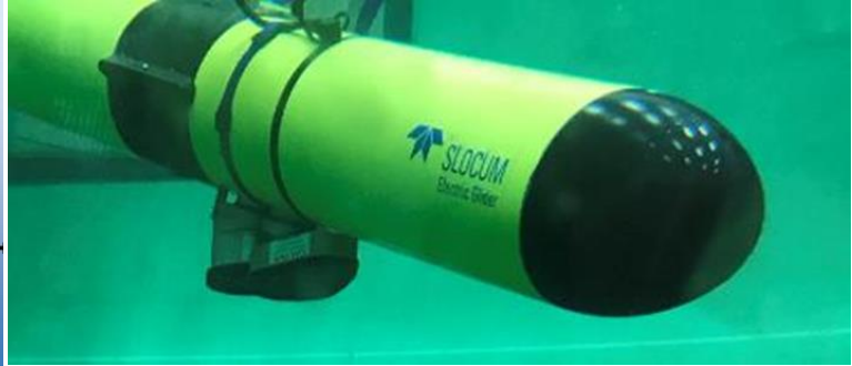
Figure 2. AZFP transducers mounted on a glider.
