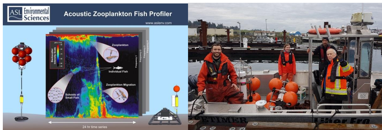
Acoustic Zooplankton Fish Profiler (AZFP) example mooring configurations and field deployment.
