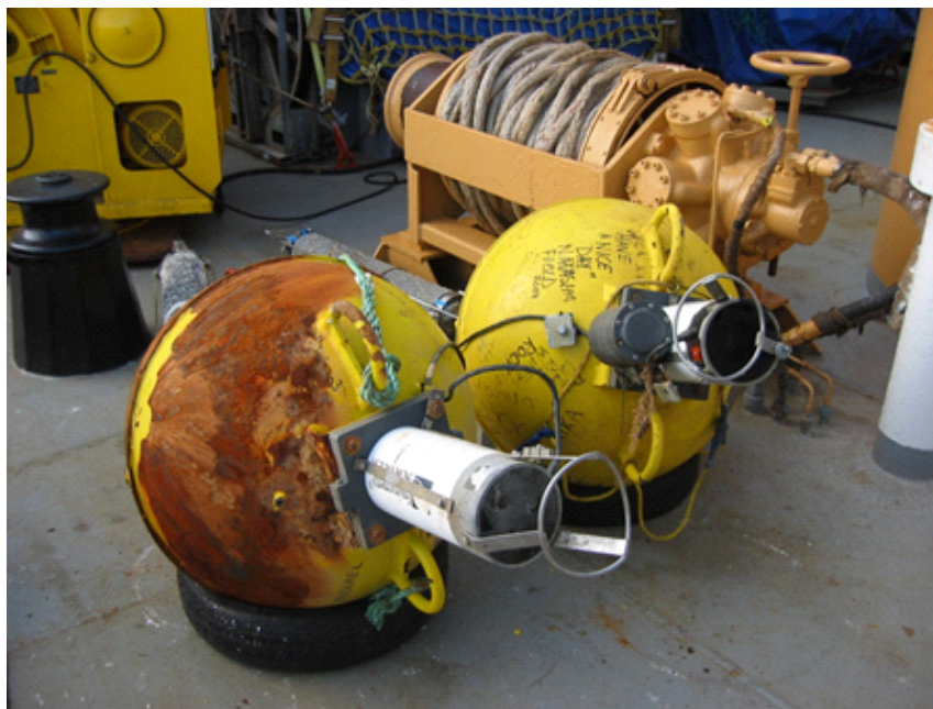
The two IPS4 units which were struck by the ice island on September 22, 2010 as seen following recovery in 2012. Besides the bent transducer guards, no significant damage was sustained.
